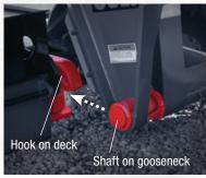
As the gooseneck approaches the deck, the **Shaft** on the gooseneck slides under the **Hook** on the deck to lift the trailer
